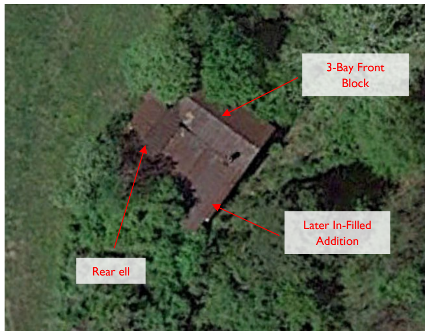
Figure 25: 2014 Google Earth aerial image of Roberta Parker Copeland House, providing clearer picture of building plan.
