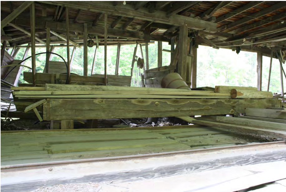
Plate 4.29: Sawmill carriage tracks which transported the logs to the saw blade on a sled.
