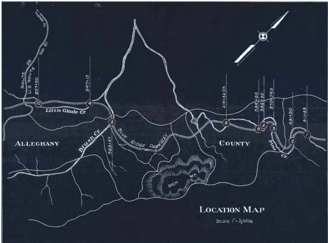
Figure 3. 1937 map showing the location of the Big Pine Creek Bridge #3 (Location 3), Big Pine Creek Bridge #6 (Location 6), and Brush Creek Bridge #1 (Location 8) (USDA BPR 1937).
