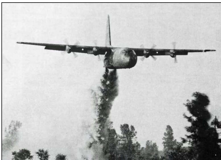
Figure 19. A NCANG MAFFS Plane in Action Dropping Fire Retardant during the 1988 Yellowstone Fire (Reid 1998:150).
