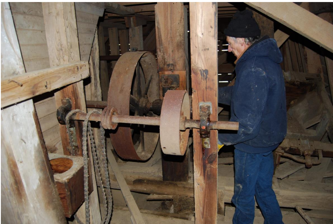
Mr. McDaniel demonstration the operation of the belt drive
