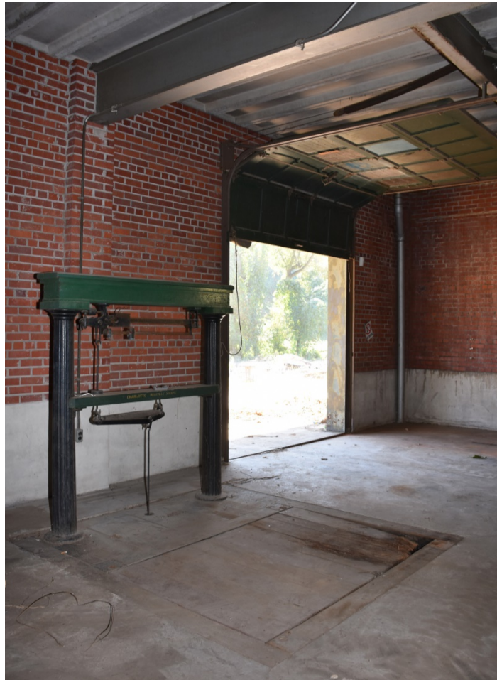
7. Freight scale near warehouse's southeast corner
